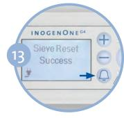
Press the alert/bell button once and screen will display "sieve reset success." Press the power button (1) to turn on the Inogen One® G4, and use normally. Press and hold the plus (+) and (-) minus buttons for 5 seconds. The screen will display "sieve reset" message. Release buttons once message is displayed on screen.
