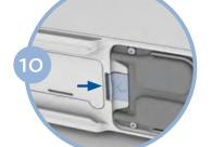
Push the column assembly into the device such that the columns are fully seated into the Inogen One® G4 concentrator. The spring loaded latch button should fully return to the closed position.
